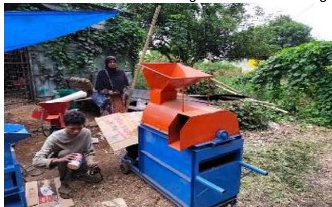
Figure 4. The Process of Assembling a Betel Nut Peeling Machine
