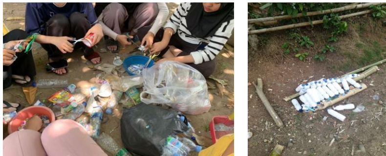
Figure 2. Cutting Plastic Waste Using Scissors, Inserting into Bottles, Compaction, Painting of Waste in Bottles
