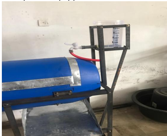
Figure 2. Bio-composter equipped with a microbial culture chamber
